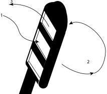
Buckle Use: The strap pushes from the back of the buckle through the middle opening, then back through the front slot allowing it to be pulled tight.
